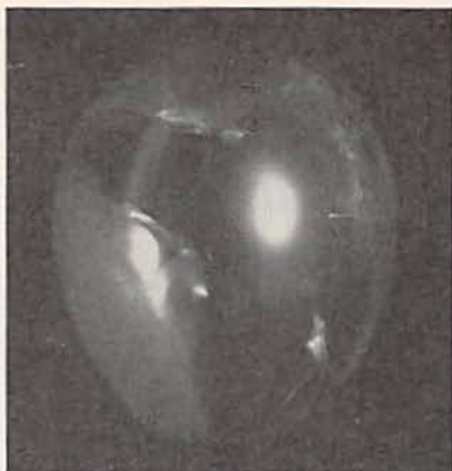
FIG. 7—AIR-FILLED BALLOON hit by a pellet. The streak on the right side is the pellet.
